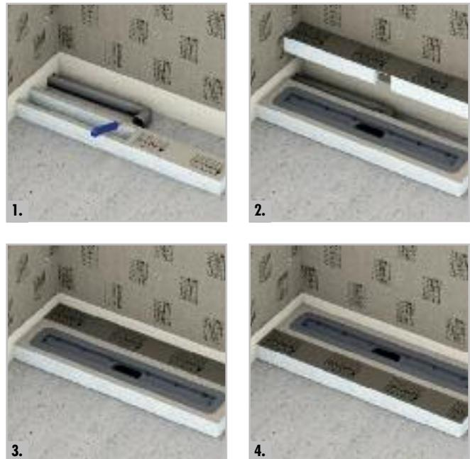
1. Depending upon the routing of the pipe, the connecting element is cut to length with a cutter / 2. After fitting the drain pipe by means of the HTK elbow, the pipe is covered safely by the connecting element / 3. + 4. Installation is possible both on the wall side and on the room side, depending on the routing of the pipe.
