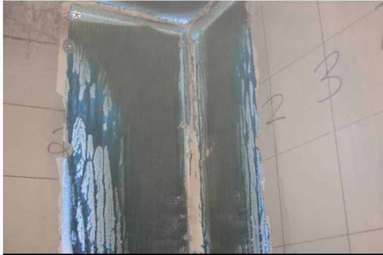
Figure 7. Post-Test View of Burn Corner Walls Near Ceiling with Foam Exposed.
