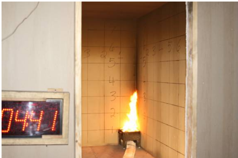
Figure 4. 4 min 41 s into Test; Burner at 40 kW.
