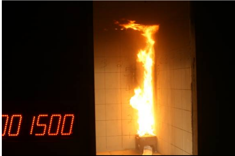
Figure 5. 15 min into Test; Burner at 160 kW; Test Completed.
