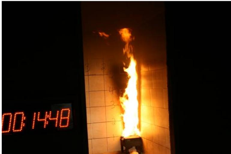
**Figure 7. 14 min 48 s into Test; Burner at 160 kW.**
