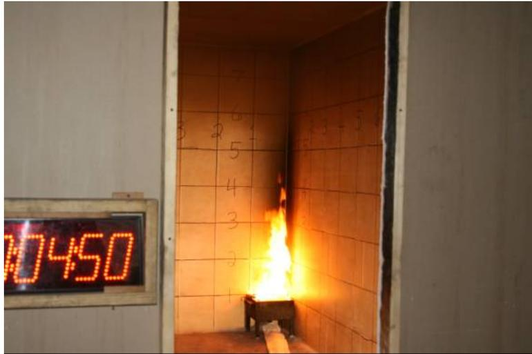
**Figure 6. 4 min 50 s into Test; Burner at 40 kW.**
